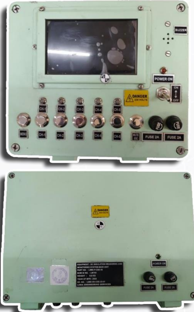
Insulation Monitoring System (IMS)
